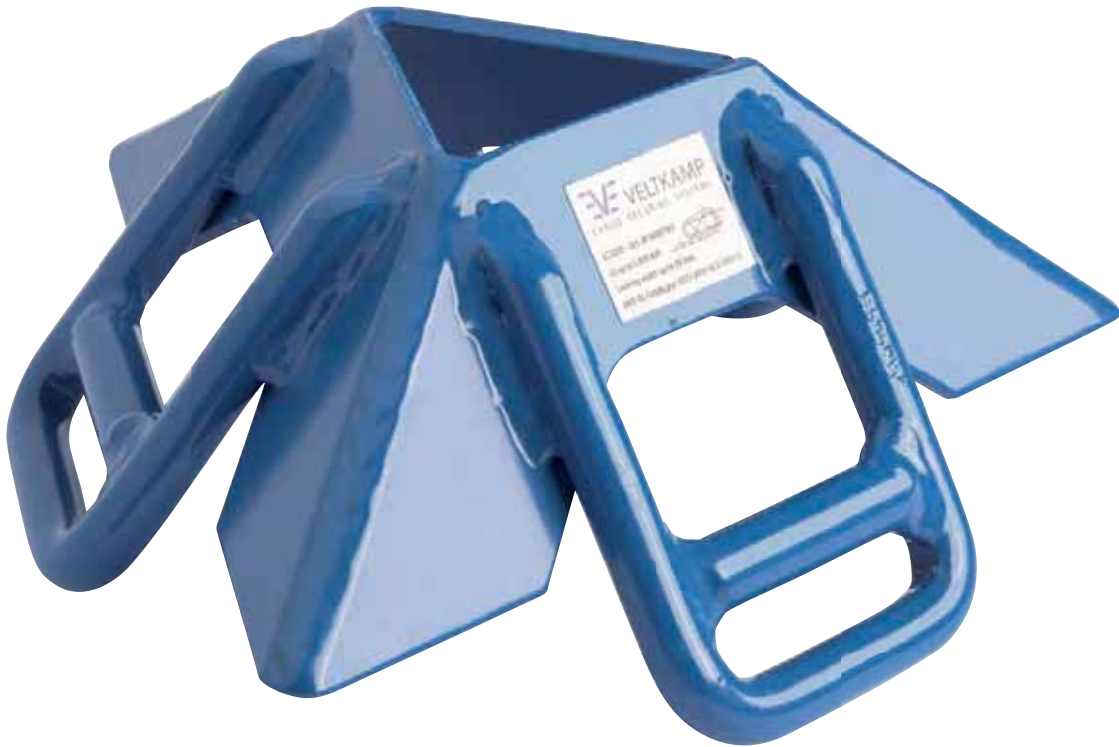
Lashing Corner LC5050 suitable for lashing up to 50mm width 210mm, height frame 60mm, total height 80mm for securing heavy crates on flatracks, trains, trucks, ships, etc.
