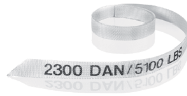
Lashing 32mm – 2,300 daN Woven Polyester – app. 250m / bag Test Certificate 4572-2014-NLD-DNV-03
