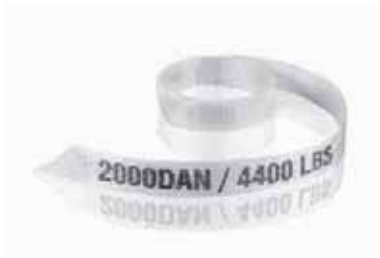
Lashing 32mm – 2,000 daN Woven Polyester – app. 250m / bag Test Certificate 4572-2014-NLD-DNV-02
